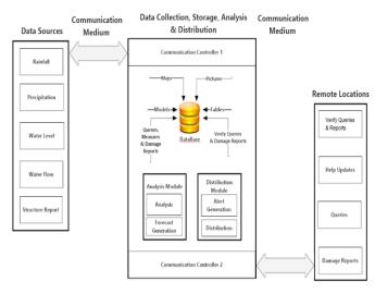
Figure 1. High-level architecture of smart flood monitoring SoS.
