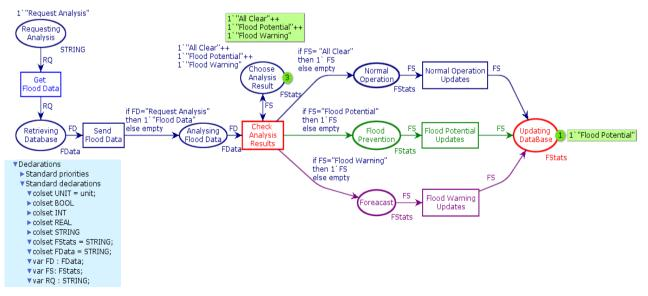
Figure 5. CPN model for flood monitoring analysis after simulation completion.
