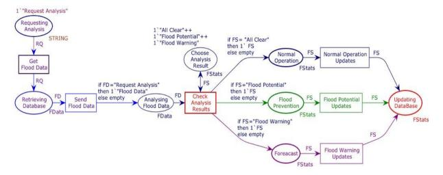
Figure 3. CPN model for flood monitoring analysis at start with tokens.
