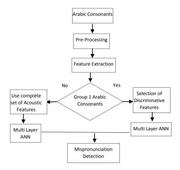
Figure 1. Proposed mispronunciation detection based on discriminative acoustic-phonetic features.
