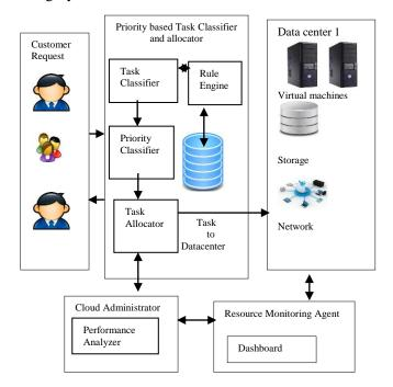
Figure 1. Architecture of cloud data center using priority queuing model.
