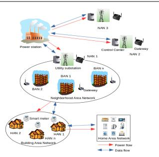
Figure 1. Communication architecture for smart grid.
