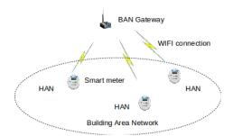
Figure 2. Smart grid architecture for AMI.
