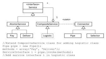
Figure 2. Modelling service structure in composite pattern.
