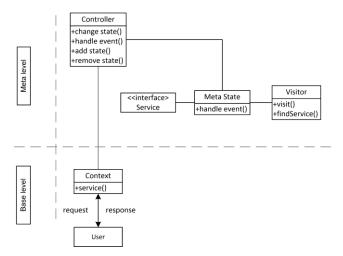
Figure 5. The reflective state pattern is used to handle user requests and provide state-dependent services.
