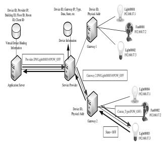
Figure 3. ID based message transmission to control actuator.
