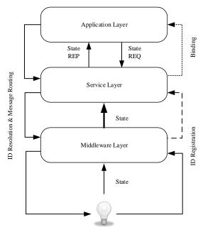
Figure 2. ID based device registration, resolution and control.
