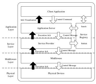
Figure 1. IoT platform for device control.
