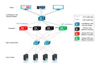
Figure 4. Load balancer architecture based on traffic pattern.
