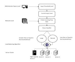
Figure 3. Load balancer architecture based on flow detection.
