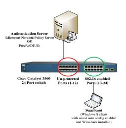
Figure 5. Test lab diagram for 802.1x wired authentication with NPS and FreeRADIUS.
