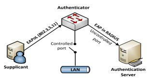
Figure 1. Components of 802.1x framework.
