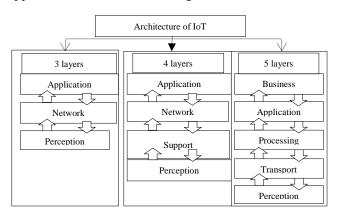
Figure 1. IoT layered architectures.
