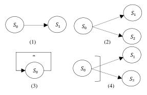
Figure 4. Structural models in service composition (sequence, parallel, loop and selection).
