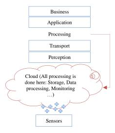
Figure 2. The relation between processing layer and the cloud.
