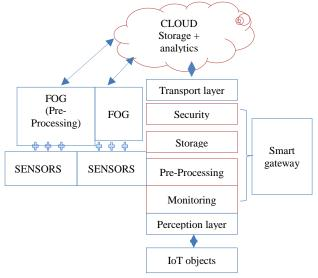
Figure 3. Cloud-Fog-IoT architecture.
