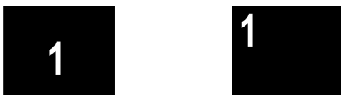
a) Translation along the x axis. b) Translation along the y axis.
