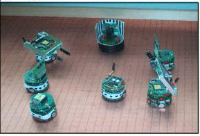
Figure 2. Seven Kheperas equipped with different devices.
