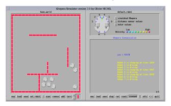
Figure 6. Snapshot of the simulation with 9 robots, in an intermediate state.
