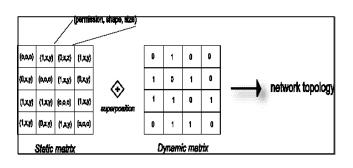
Figure 4. Superposition of the dynamic and the static matrices.
