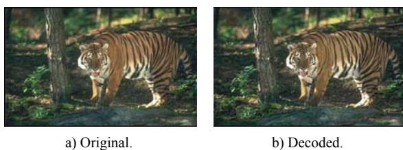
Figure 16. System results (PSNR=35.63, MSE=13.9, CM=0.8, CR=0.131).
