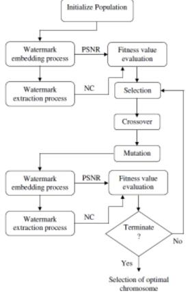
Figure 5. Technique using GA.
