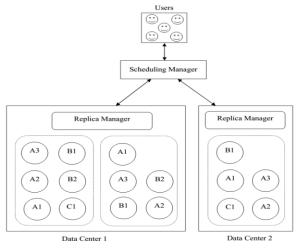
Figure 2. Sample cloud data center architecture.
