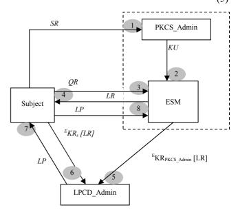
Figure 7. ESM: Subject query request and label permit process, where numbered arrows illustrate the secrecy and authentication stages.
