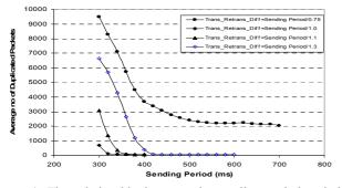
Figure 4. The relationship between the sending period and the average number of duplicated packets at different time difference between the transmission and retransmission messages.
