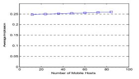
Figure 10. The relationship between the average implosion and the no. of receiver when the sending period is equal to 340 ms.
