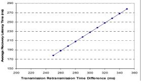
Figure 12. The effect of changing the time difference between the transmission and retransmission messages and the average recovery latency time.
