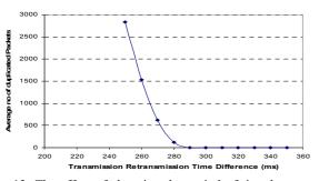
Figure 13. The effect of changing the period of time between the transmission and retransmission messages on the average no. of duplicated packets.
