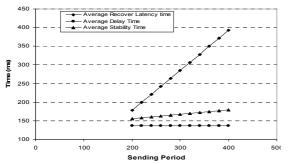
Figure 5. The effect of the sending period on the average (recovery latency, delay, and stability) times.
