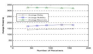
Figure 11. The effect of the no. of receivers on the different average times when the sending period is equal to 340 ms.
