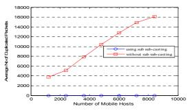
Figure 9. The relationship between the average no. of duplicated packets and the no. of mobile hosts when the sending period is equal to 340 ms.
