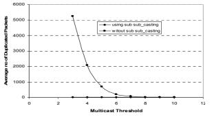
Figure 7. The relationship between the multicast threshold and average no. of duplicated packets.
