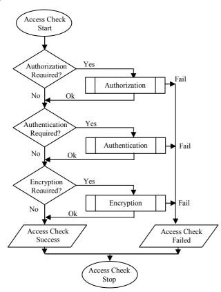
Figure 3. Access check flowchart.
