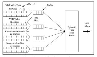
Figure 3. ATM simulation model.
