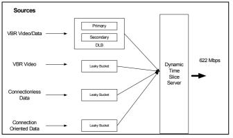
Figure 2. DLB in ATM switch.
