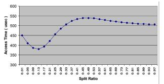
Figure 4. The access time of the simulated database versus split ratio.
