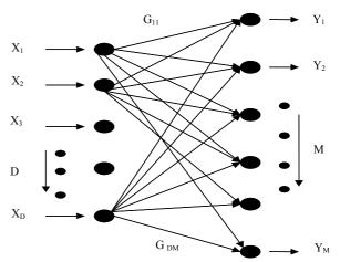
Figure 4. Topology of the neural network used in the hybrid NN-DVQ configuration.
