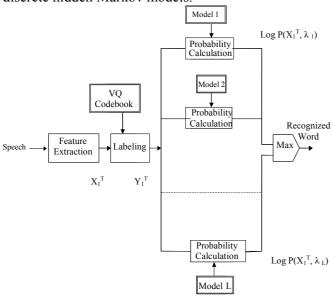
Figure 1. Schematic diagram of the VQ/HMM isolated word recognition system.
