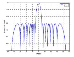
Figure 2. Comparison of the radiation patterns of the broad side linear array with excitation coefficients by the Chebycheff and the TS method.
