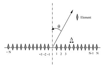
Figure 1. Equdistant elements symmetrical linear array .
