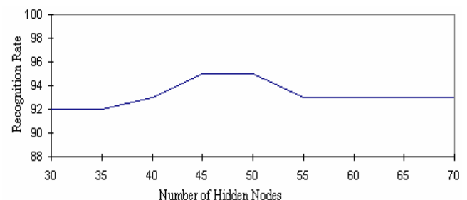
Figure 10. Graph of recognition rate versus number of hidden nodes.
