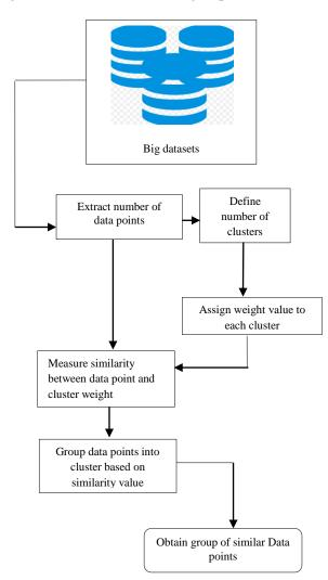
Figure 1. Architecture diagram of the SDI-WIXC technique.
