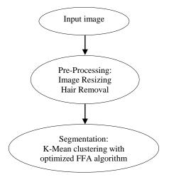
Figure 1. Framework of the proposed segmentation technique.
