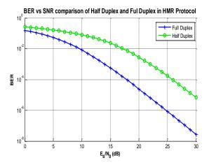
Figure 5. BER vs EB/No performance of half duplex and full duplex in HMR Protocol.
