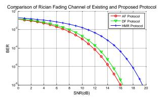
Figure 11. Comparison of rician fading channel with existing protocol and proposed HMR protocol.
