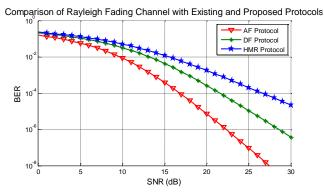
Figure 10. Comparison of rayleigh fading channel with existing protocols and proposed HMR protocol.
