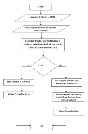
Figure 4. An operational flowchart of HMR protocol.
