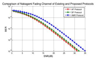
Figure 12. Comparison of nakagami fading channel with existing protocols and proposed HMR protocol.
