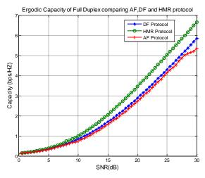
Figure 9. Ergodic Capacity of full duplex comparing AF, DF, and proposed HMR protocol.
