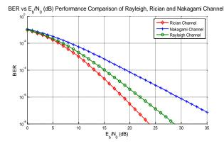
Figure 13. BER vs EB/No performance comparison of rayleigh, rician and nakagami channel.
