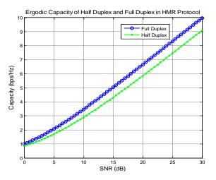
Figure 8. Ergodic Capacity of half duplex and full duplex in HMR protocol.
