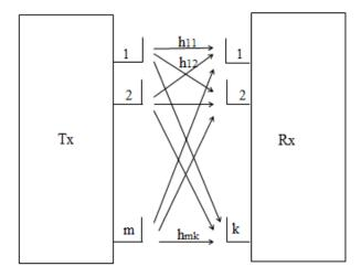
Figure 1. MIMO system model.
