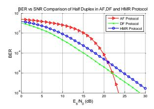
Figure 6. BER vs SNR Comparison of Half Duplex in AF, DF and proposed HMR Protocol.
