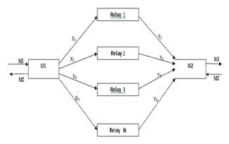
Figure 3. Half duplex and full duplex relay system.
