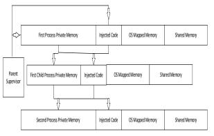
Figuer 2. Process chaining control diagram.
