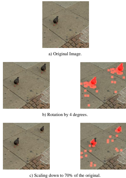
Figure 4. Detecting forgeries under rotation and scaling. Left images are the forged images. Right images are the forged images after being detected.
