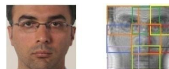
Figure 6. The original and the corresponding Fresnel transformed image divided into 3x3 overlapping regions.
