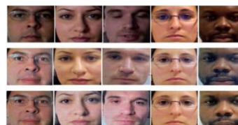
Figure 2. Example of PRINT-ATTACK database images, real faces (upper row) and from printed photos with the glued photograph (middle row) and hand held ones (lower row). As we can see there are many similarities that make it hard to separate real pictures from the fake ones.
